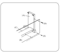
**3.** Place the piano on the front half of the stand so that the metal fitting holes are seen when viewed from the top. Slide the piano backward while holding it with one hand so that it does not incline and fall from the stand. The hooks on the piano are then engaged with the metal fittings on the Side Panels. Pay attention so that hands or fingers are not caught between the stand and piano.
