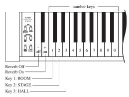
The REVERB function is automatically activated when the CN22 digital piano is turned on.
